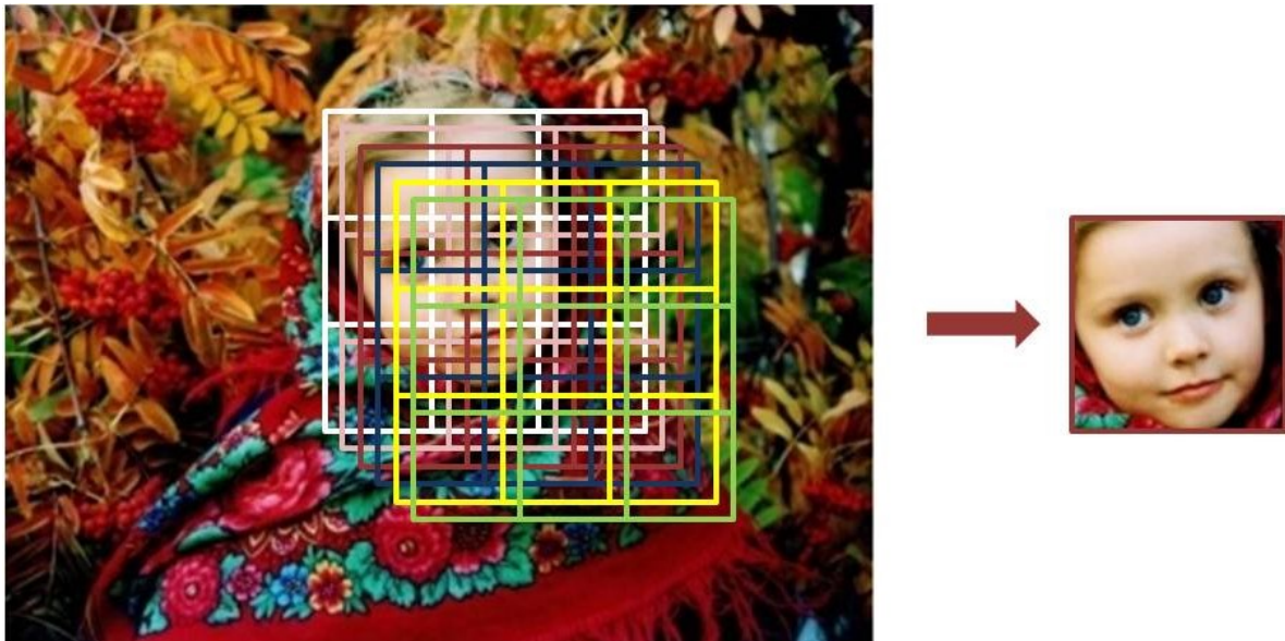
Figure 4. Few sparse systems of frames with offsets. The third system includes the frame, for which Cascade Classifier returns positive result
